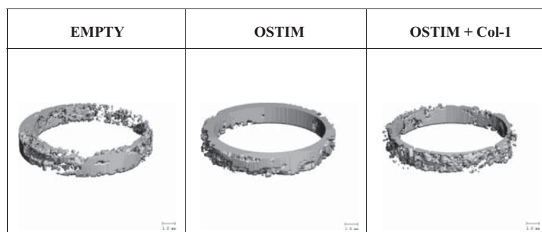
Fig. 1. 3D reconstructed images of the region of interest for high-resolution peripheral quantitative computed tomography (HR-pQCT) of the defective bone sites representing a ring shaped hollow cylinder with 1 mm offset thickness and 2 mm in depth at the host bone-defect/biomaterial interface.
