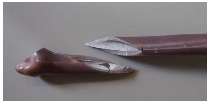
Fig. 2. Fourth generation sawbone model after osteotomy of the femoral neck and creation of a standardized characteristic 14 cm spiral fracture using a template and milling machine.
