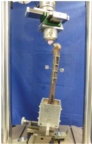
Fig. 4. Test setup for cyclic fatigue testing of periprosthetic fracture fixation using a servo-hydraulic testing machine (Instron 8874, Instron Ltd., High Wycombe, UK).
